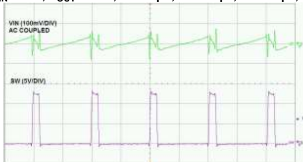
Time- 1µs/div Input Voltage Ripple
