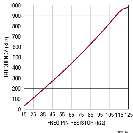
Figure 2. Switching Frequency vs Resistor on FREQ pin
