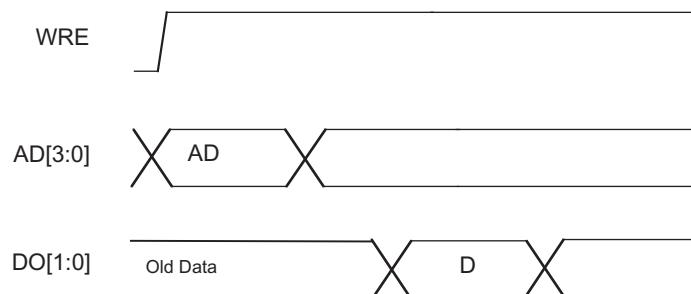
Figure 3-8. Slice Single /Dual Port Read Cycle Timing
