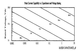
These are typical curves for KV<sup>X</sup> capacitors with mica-paper dielectric. Other dielectric systems are available with improved characteristics. Please contact us for information.
