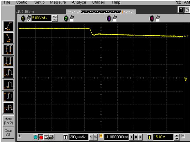
FIGURE 10. VLN TRANSITIONS FROM 18.3V TO 13.3V
