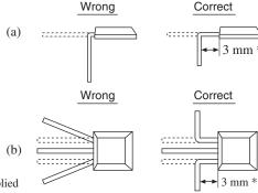
Bending position of lead wire
