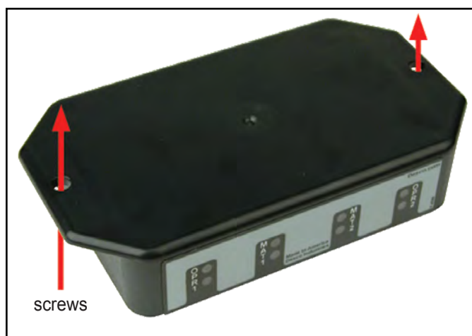
Figure 2. Mounting the Control Unit
