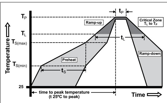
Wave Soldering      260°C, 10 seconds max.
