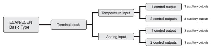
Note: Models with one control output or two control outputs can be used for heating/cooling control.
