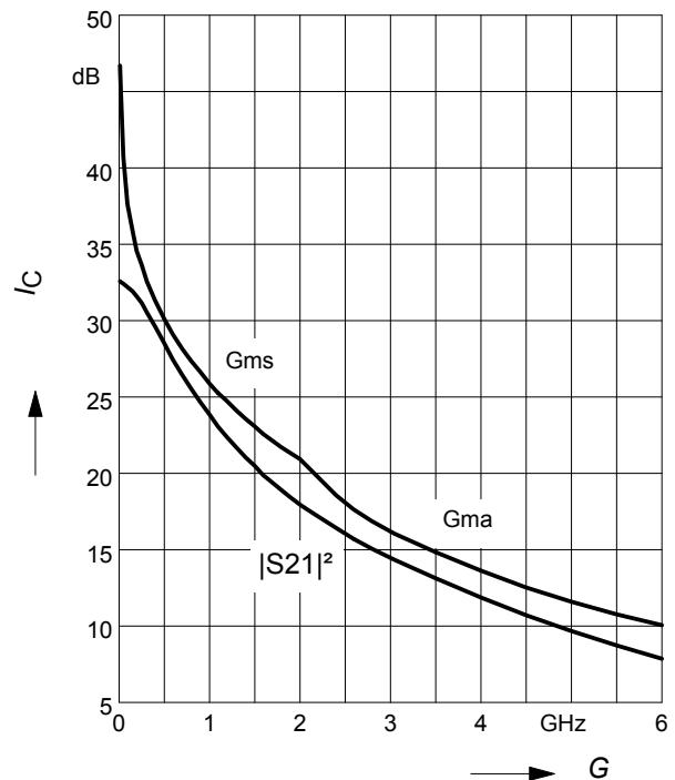
**Power gain  $G_{\text{ma}}, G_{\text{ms}} = f(V_{\text{CE}})$**
