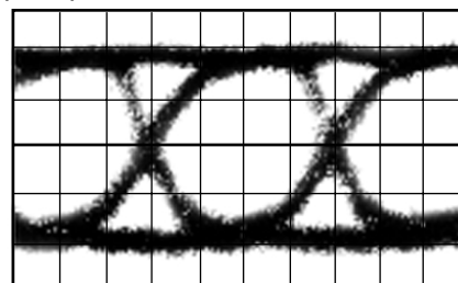
Fig.4 Eye Diagram with a 1,550nm, 2.5Gb/s NRZ, 2^{23}-1 PRBS incident signal
