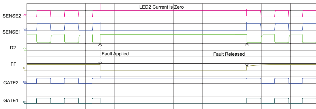
Figure 2A: Drain Short-to- V_{IN} Fault on D2 with \text{MODE} = \text{HIGH} and PWM Dimming
