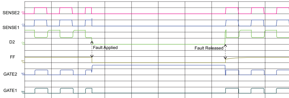
Figure 4A: Open-LED Fault on D2 with MODE = HIGH and PWM Dimming
