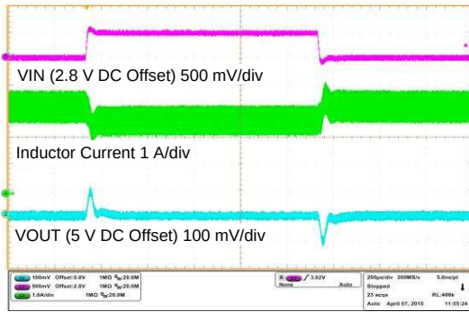
VIN = 2.8 V to 3.3 V, VOUT = 5 V, IOUT = 2 A
