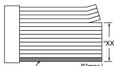
Breakout starts with Number 1 lead indicated by brown wire or red stripe. Shown on top side.
