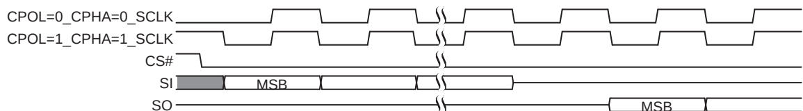
Figure 4.1 SPI SDR Modes Supported
