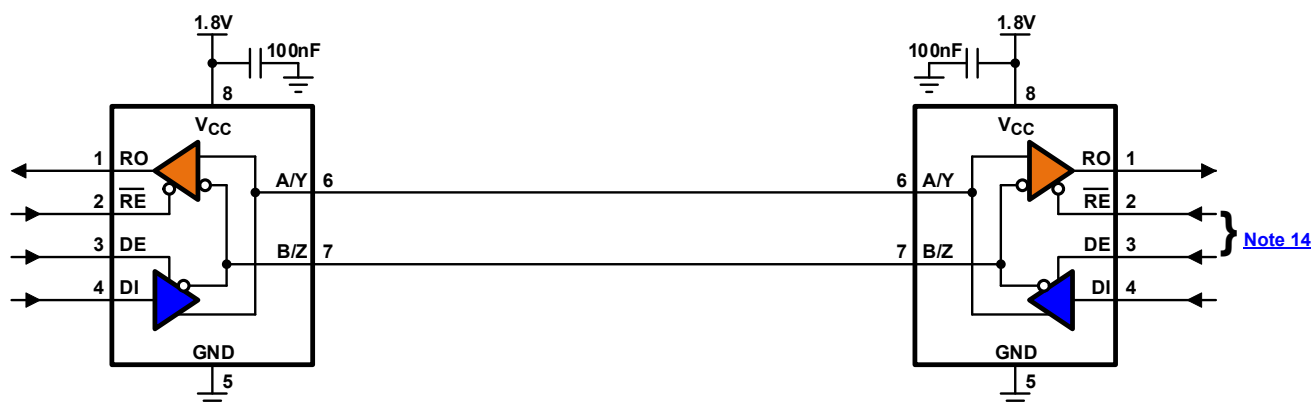
FIGURE 3. HALF DUPLEX NETWORK USING ISL32603E
