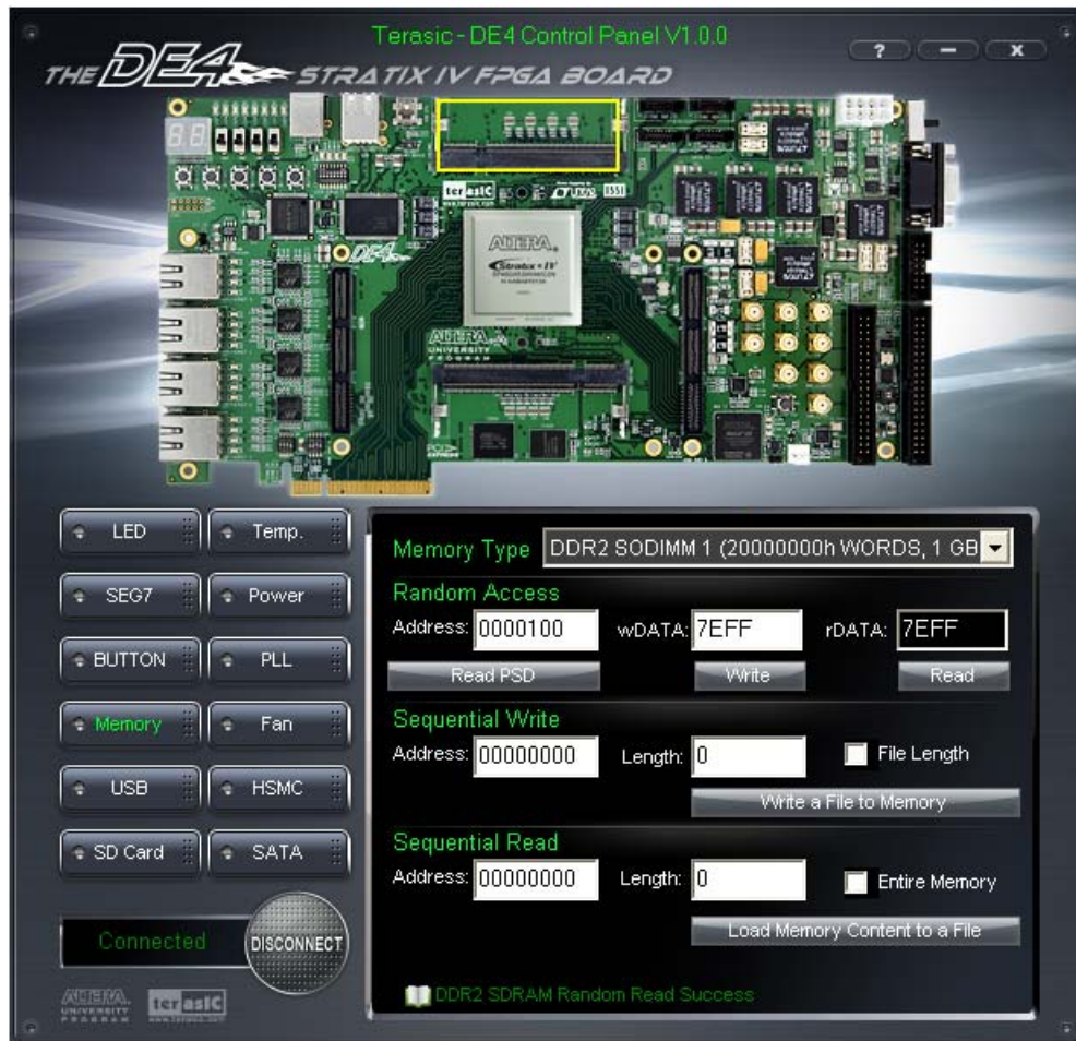
Figure 3–9 Writing the hexadecimal value 7EFF to location 0x100
