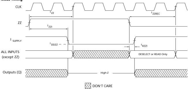
21. Device must be deselected when entering ZZ mode. See Cycle Descriptions table for all possible signal conditions to deselect the device. 22. DQs are in High-Z when exiting ZZ sleep mode.
