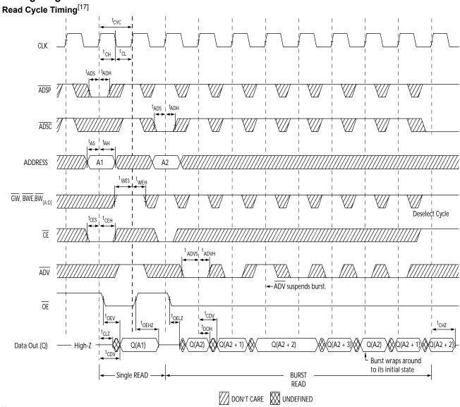
Note: 17. On this diagram, when  $\overline{CE}$  is LOW,  $\overline{CE}_1$  is LOW,  $\overline{CE}_2$  is HIGH and  $\overline{CE}_3$  is LOW. When  $\overline{CE}$  is HIGH,  $\overline{CE}_1$  is HIGH or  $\overline{CE}_2$  is LOW or  $\overline{CE}_3$  is HIGH.
