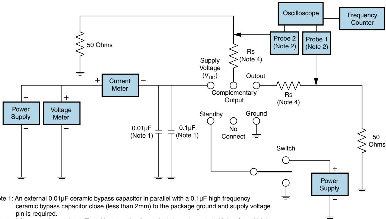
Note 1: An external  $0.01\mu\text{F}$  ceramic bypass capacitor in parallel with a  $0.1\mu\text{F}$  high frequency ceramic bypass capacitor close (less than 2mm) to the package ground and supply voltage pin is required.
