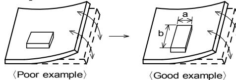
Products shall be located sideways (Length:a<b) to the mechanical stress.
