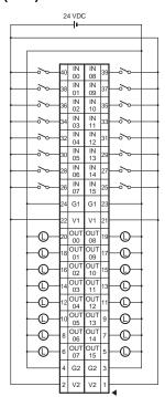
**Screw-less Clamp Terminals with Transistors**
