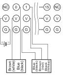
Two-wire sensor Three-wire sensor with PNP output (e.g., photoelectric sensor or proximity sensor)
