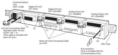
**Note:** The connecting cable for the I/O Unit is shown below. Accessory Cable
