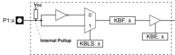
**Figure 28. Keyboard Input Circuitry**
