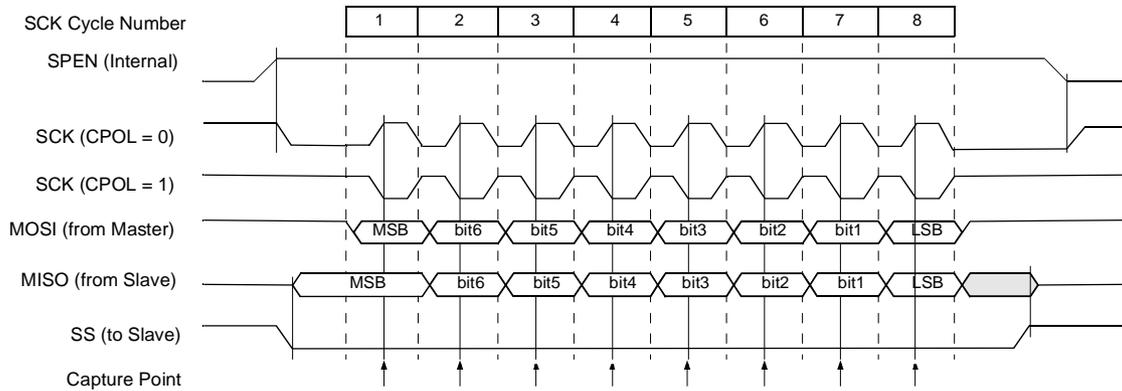
**Figure 40. Data Transmission Format (CPHA = 1)**
