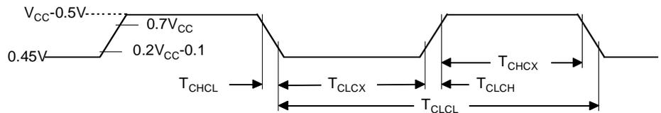
**AC Testing Input/Output Waveforms**
