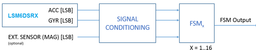
Figure 2. State machine in the LSM6DSRX
