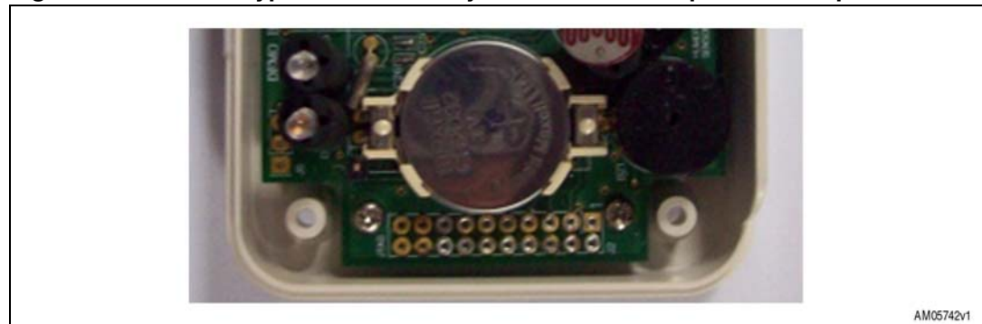
Figure 58. 3 V coin-type CR2032 battery insertion for RTC power backup
