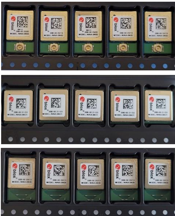
Figure 9: Orientation of NINA-B410/B411/B416 modules on tape
