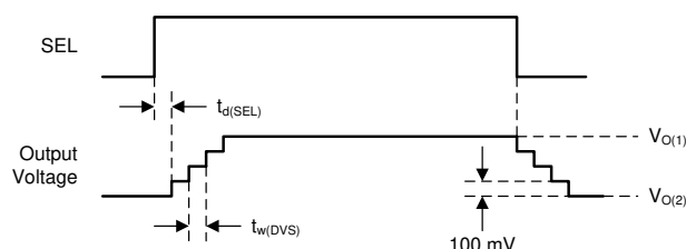
Figure 7-10. Dynamic Voltage Scaling with High Load
