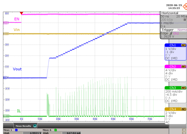
Figure 8-28. Start-up Behavior from Rising Enable
