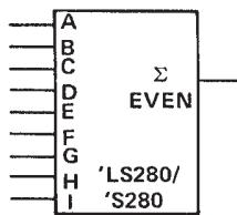
As an alternative, the outputs of two or three parity generators/checkers can be decoded with a 2-input ('S86' or 'S135') or 3-input ('S135') exclusive-OR gate for 18- or 27-line parity applications.
