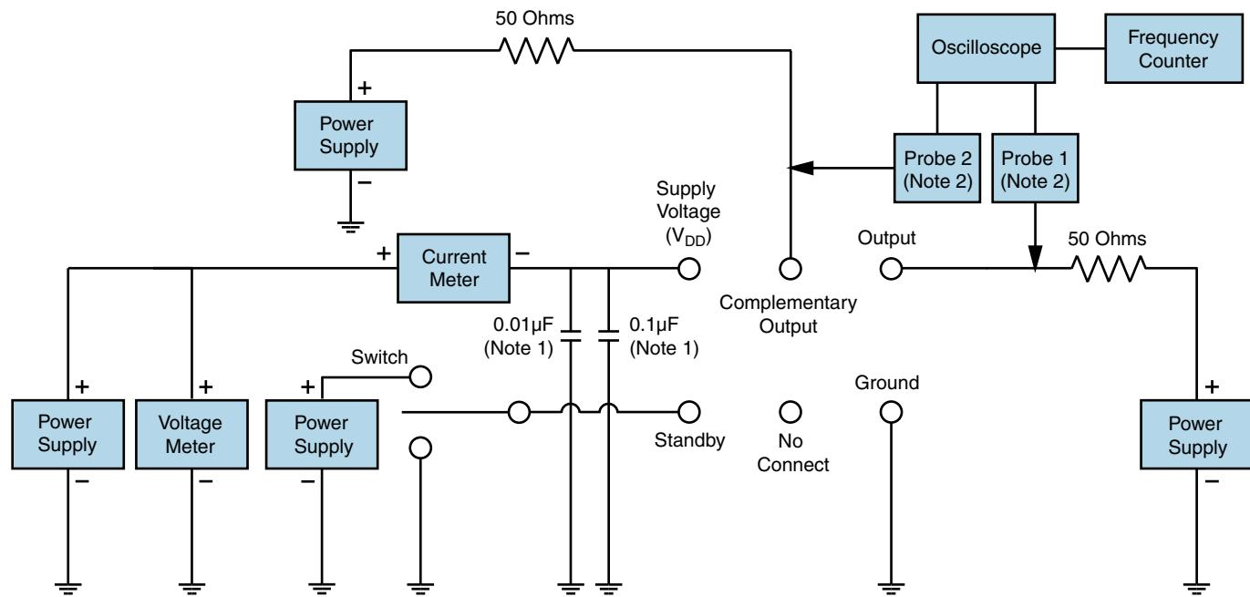
Note 1: An external  $0.01\mu\text{F}$  ceramic bypass capacitor in parallel with a  $0.1\mu\text{F}$  high frequency ceramic bypass capacitor close (less than 2mm) to the package ground and supply voltage pin is required.
