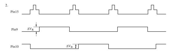
Input 100 % white signal and adjust the voltage of Pin4 so that  $\Delta V_B$  becomes 0 mV. Let the adjusted voltage be  $V_{AD4}$ .
