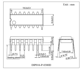
Note) The package of this product will be changed to lead-free type (DIP016-P-0300M). See the new package dimensions section later of this datasheet.
