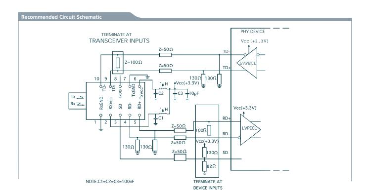
The split-load terminations for ECL signals need to be located at the input of devices receiving those ECL signals. The power supply filtering is required for good EMI performance. Use short tracks from the inductor L1/L2 to the module  $R_X$   $V_{CC}$  and  $T_X$   $V_{CC}$ . A GND plane under the module is required for good EMI and sensitivity performance.
