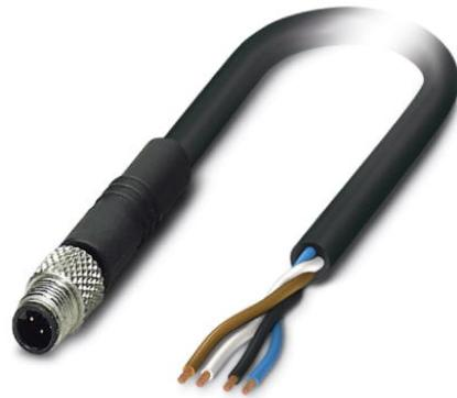
Sensor/Actuator cable, 4-position, PUR, Black RAL 9005, Plug, straightLink:M5, A-coded, on Free conductor end, Cable length: 1.5 m
