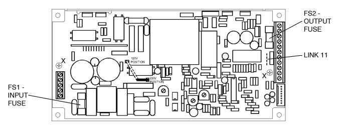
The input fuse is also accessed by removing the cover, as above.
