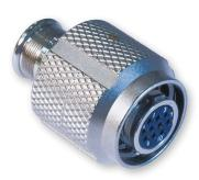
Series 805 Plugs: feature two shell styles including and Integral platform for direct shield attachment using Band-Master™ ATS termination system or accessory thread for attaching a connector backshell for strain relief. EMI ground spring achieves low shell-to-shell resistance. This nickel-plated beryllium copper spring enables the Series 805 to meet greater than 60 dB
