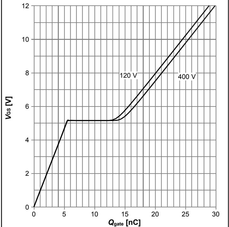
$V_{GS}=f(Q_{gate})$ ;  $I_D=5.6$  A pulsed; parameter:  $V_{DD}$
