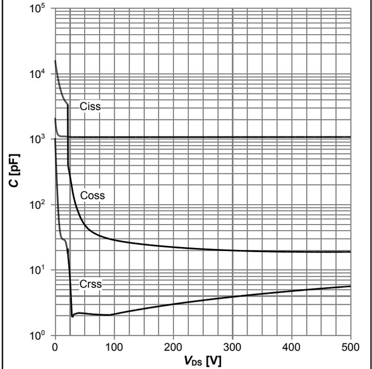
$C=f(V_{DS}); V_{GS}=0 \text{ V}; f=250 \text{ kHz}$
