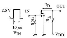
$V_{DD} = 3 V$   $D.U. \le 1\%$   $V_{IN}: t_r, t_f < 5 \text{ ns}$   $(Z_{out} = 50 \Omega)$  COMMON SOURCE  $Ta = 25^{\circ}C$
