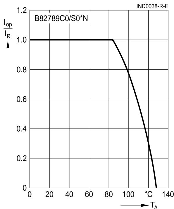
Current derating  $I_{op}/I_R$  versus ambient temperature (rated temperature  $T_R = 110^\circ\text{C}$ )
