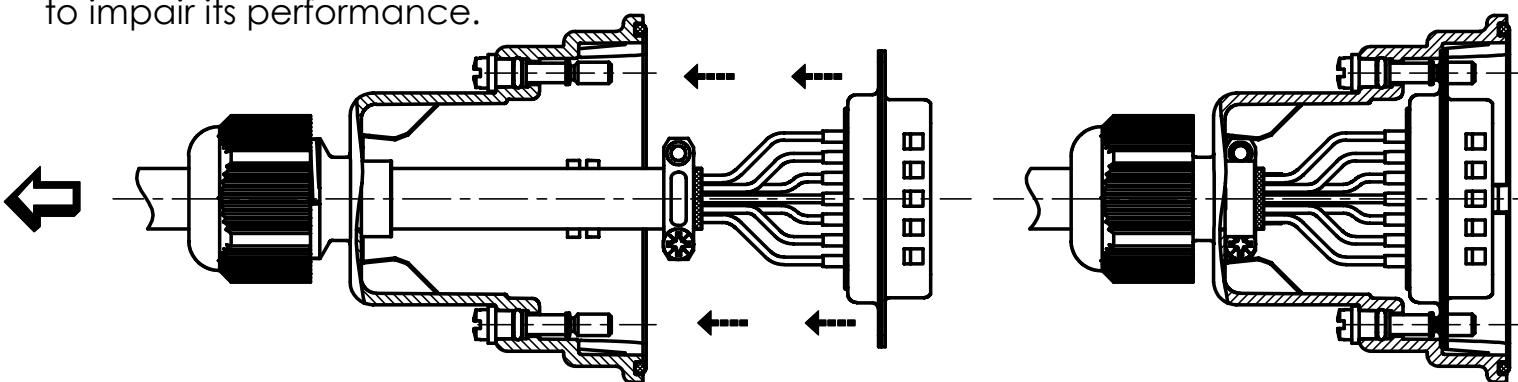
Pull back cable until cable clamp snaps into shielding plate. Snap connector into hood.
