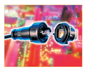
Coupling ring, screw thread protection against damage provides secure cable coupling through mis-use and positive alignment for mating of connectors Panel gasket maintains IP68 seal to panel Sealing gland and cage optimised to maintain IP68 seal and provide secure cable restraint without disrupting signal 'O' ring maintains IP68 seal Shielded Cat 5e coupler at connector interface maintains screening
