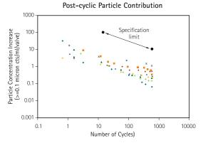
Note: After cycling the valves for 2.1 M cycles in 49  $\pm$ 3% HF, the valves must also pass the particle contribution criteria.
