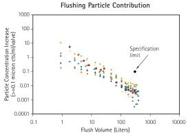
Note: During initial flushing, the device must contribute <0.1 particle/ml (particle size  $\geq$ 0.1  $\mu$ m) within 300 liters of flushing. During operation, the device must release <100 particles/actuation (particles size  $\geq$ 0.1  $\mu$ m) within 500 cycles and <10 particles/actuation (particles size  $\geq$ 0.1  $\mu$ m) within 10000 cycles.
