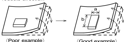
Products shall be located in the sideways direction (Length: $a < b$ ) to the mechanical stress.
