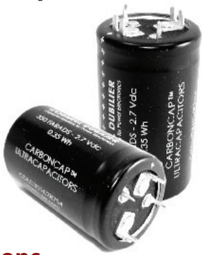
This leading edge, organic electrolyte D cell ultracapacitor can easily handle more than a half million duty cycles and has multiple pins and snap-in terminals for easy, reverse proof, robust, board mounting. They are suited for industrial power back up, renewable energy systems, short term UPS, and telecom applications.
