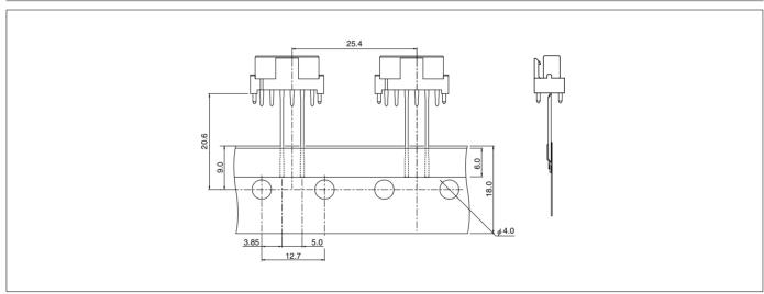
Note: Conforms to JIC C 0806 of "Tape packaging of components with unidirectional leads on continuous tapes".
