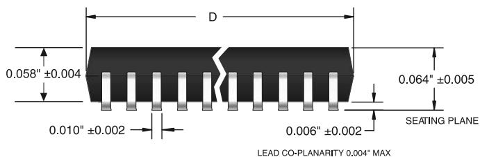
Note: All dimensions exclude mold flash and end flash which shall not exceed 0.006" per side.
