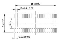
Recommended solder paste thickness: 120  $\mu$ m
