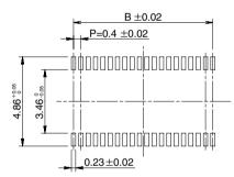
Recommended solder paste thickness: 120  $\mu$ m
