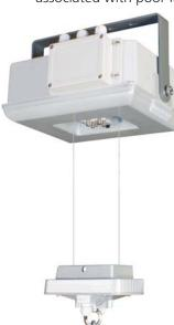
As soon as the lift is lowered, power is automatically cut off to the luminaire allowing maintenance to be carried out safely and easily. When the luminaire is raised back to its original docking position, power is automatically restored with immediate illumination.
