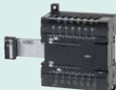
CP1W-16ER Relay outputs: 16
