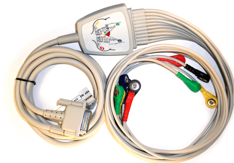
Figure 48. 15-Pin, Shielded Connector from Biometric Cables
