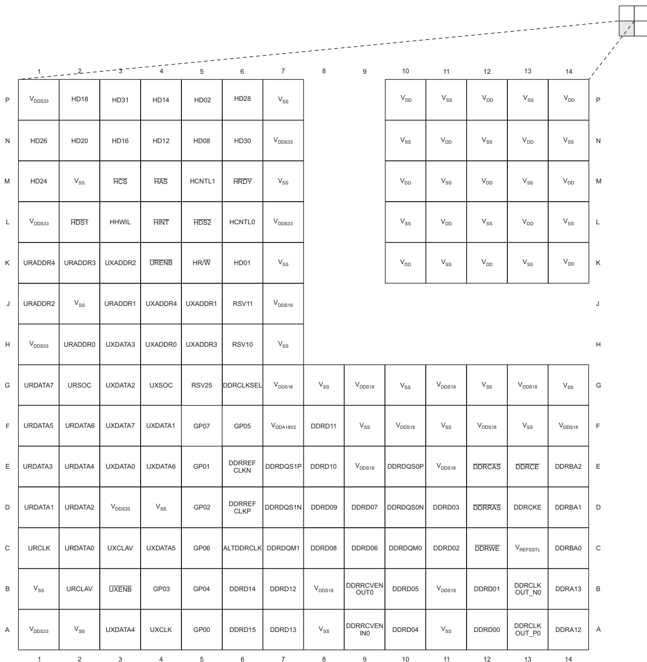
Figure 2-5 TMS320C6457 Pin Map (Bottom View) [Quadrant D]
