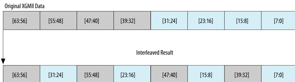
Figure 6-5: Interleaved SDR XGMII Data Mapping
