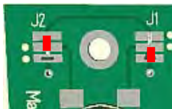
Solder pads J_1 and J_2 connection for reversed heat flux direction
